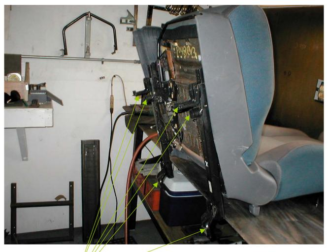
Drill rivets and grind welds clean to remove original mounting brackets (3 on each side).
