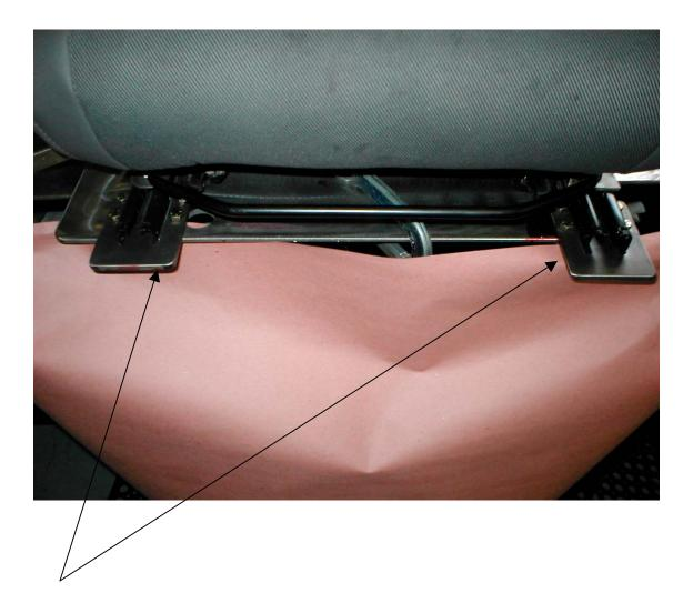
Slide seat into rear track retainers and attach front track retainers as shown. Once front track retainers are installed, check to be sure seat tracks are as far forward as the front retainers will allow. Then drill ¼" hole through seat tracks from bottom, using hole provided in seat mounting plate as a locator. Use ¼-20x1 button-head bolts (provided).
