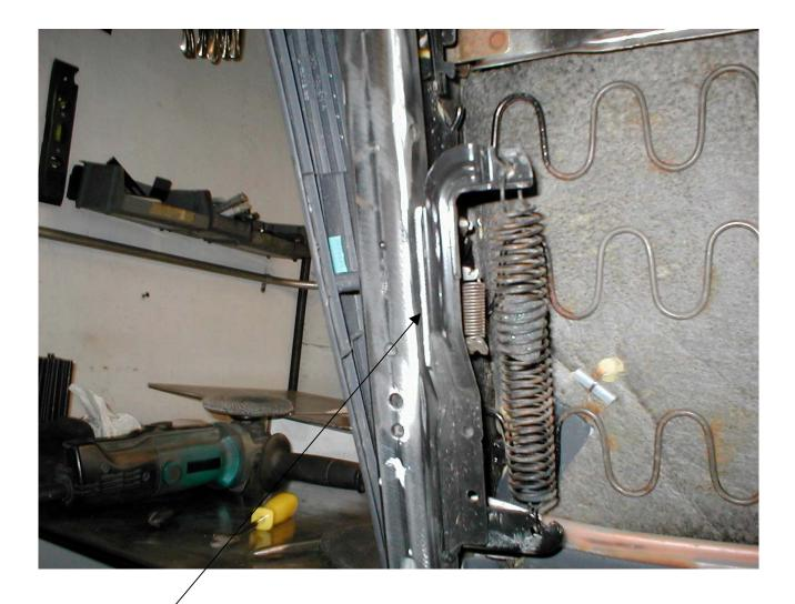
Grind front spring mounting brackets here so they do not protrude below seat tracks (Both sides).
