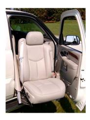
The EASY REACH brings your existing seat completely outside the vehicle and down toward the ground to an easy transfer height for maximum convenience. Once transferred, you ride up into the vehicle and rotate forward for a smooth, comfortable and safe ride in your vehicle's original seat.
