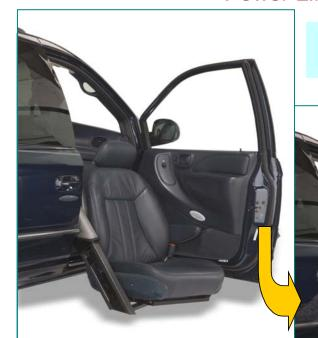
Seat glides completely outside vehicle and to ground for convenient transfers
